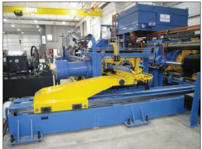
Figure 5. Billet loading on the Tecalex 2,200 U.S. ton super-compact press in operation at plant #4.
