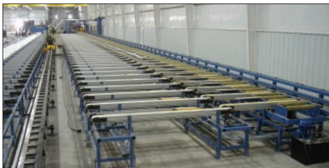
Figure 7. Tecalex puller in operation at plant #4.
