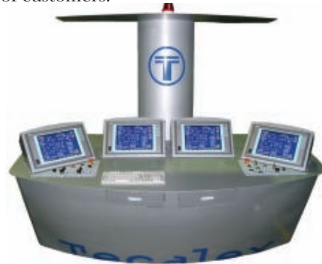
Figure 8. SCADA production system at plant #4.
